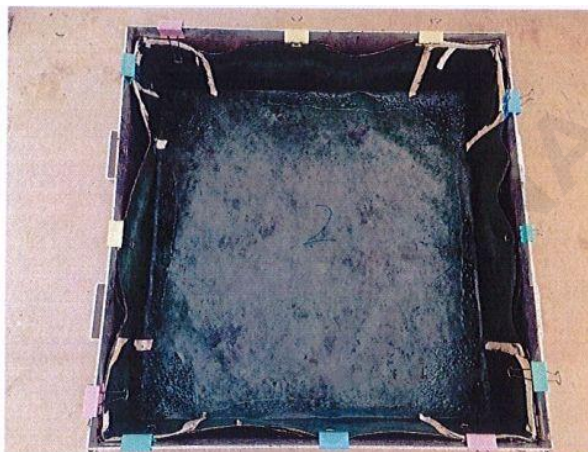
Photos of Coating Surface and Corners for Test Box No. 2
